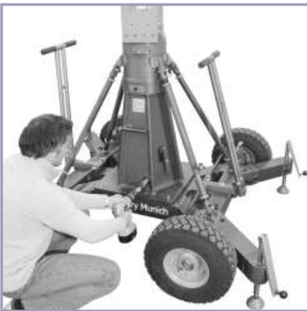
Retracted column for transport and assembly
